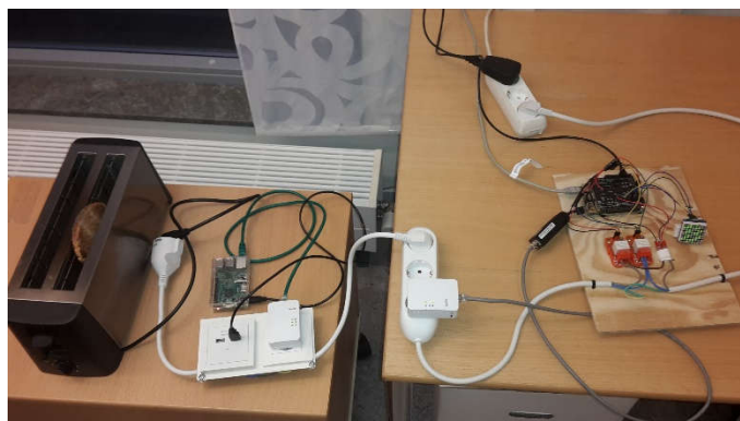
Fig. 5. The prototype implementation. The smart cable to the left connected plugged into the smart socket system to the right.
